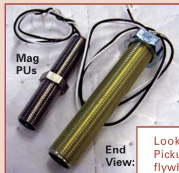
The same in all other respects, different-sized Mag pickups take a different size mounting hole in the flywheel housing.
