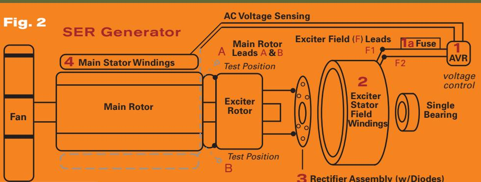
Lastly, to check the generator windings (Lines 1, 2, 3, & Neutral), check voltage between three legs first, then from each leg to neutral. Should be 120 V line-to-neutral.
