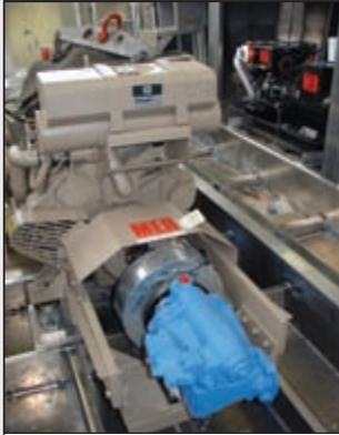
MER MG8.8 kW Isuzu genset; custom hydraulics on the Deere run propulsion jets for vessel's shallow draft.
