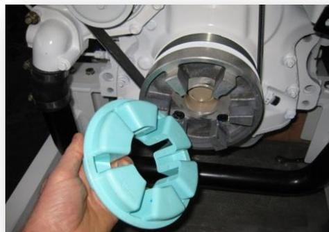
Figure 7: Insert the elastomeric insert, into the coupling.
