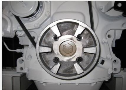
Figure 6: Bolt the other half of the coupling to the front of the crank, using thread-locking compound and tightening the bolts to 50 ft/lb.
