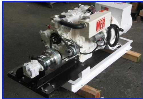
Figure 3: Here the hydraulic pump is on the front and the generator on the rear.
