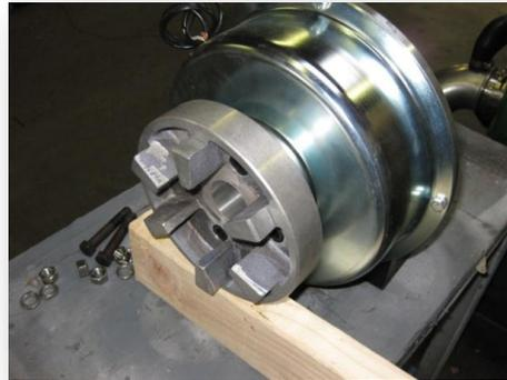
Figure 5: Begin by bolting one half of the MER-Drive coupling to the clutch assembly. Use lock washers when needed, apply thread-locking compound to the bolts, and tighten to 50 ft/lb.
