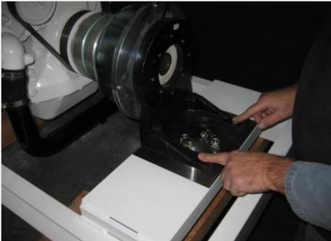
Figure 10: Install the clutch mounting feet bolts, and temporarily snug them to approximately 30 ft/lb.
