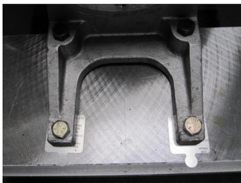
Figure 11: If the clutch side of the coupling is higher than the engine side by more than .010", and there are no shims which can be removed from beneath the clutch pad, then the engine must be shimmed up to match the clutch side. For example, if the clutch-side coupling is higher than the engine side by .020", then add the .020" of shims to each of the four engine mounting feet.
