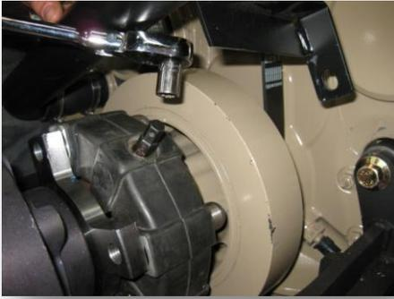
**Figure 5** Begin by removing the radial bolts from the torsional coupling.
