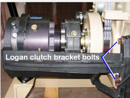
**Figure 7** Remove the bolts securing the clutch bracket to the engine block. Now slide the clutch bracket and clutch forward until there is adequate
