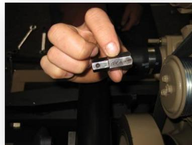
Figure 4 The 14MM Allen head, drive pin removal tool is available from MER Parts.
