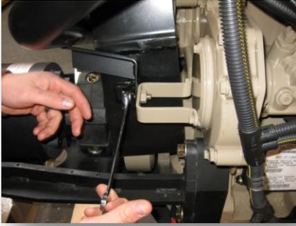
Figure 10 Next remove the fasteners that secure the grill-type belt guard shown here. This includes the bolt that connects the belt guard and coolant cross-over tube to the U-shaped bracket that is tan in color.
