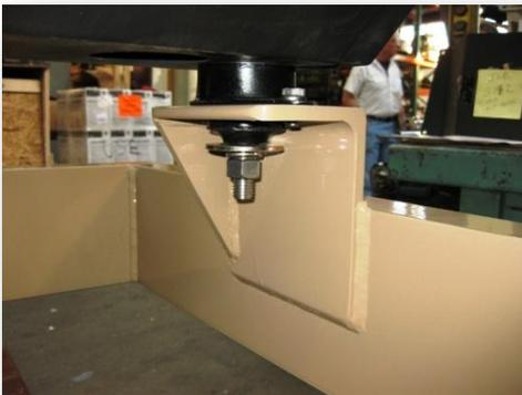
Figure 1 Remove the 5/8" bolt securing the isolation mount to the black clutch bracket.
