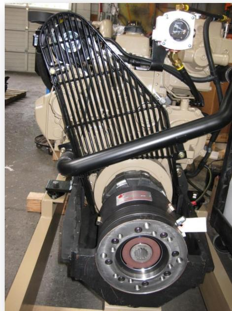
**Figure 9** MER/Deere engine with Logan front mounted PTO clutch.
