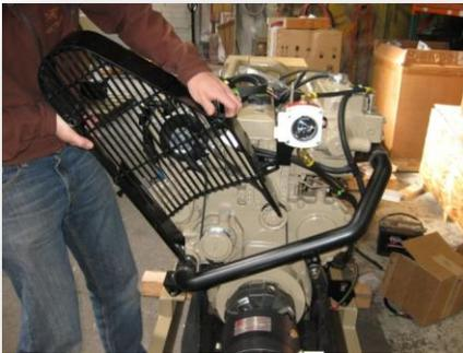
Figure 11 Remove the pound belt guard from its position.
